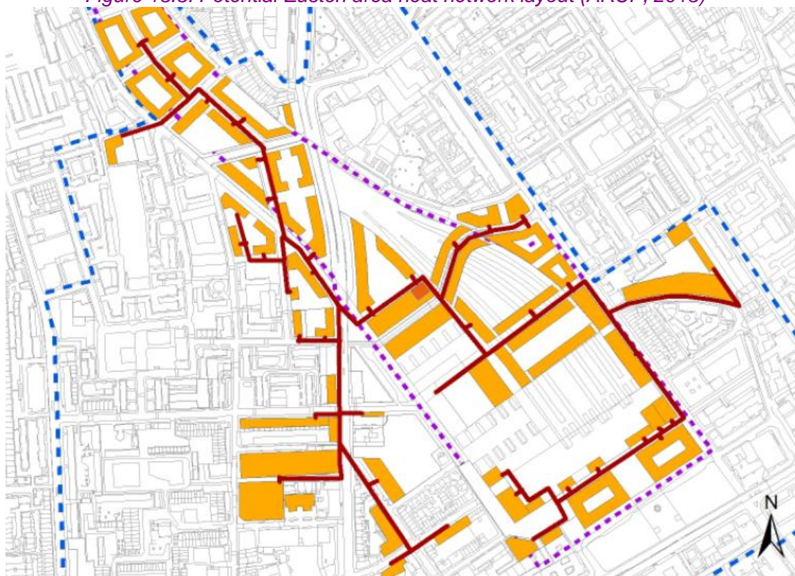
Figure 13.3: Potential Euston area heat network layout (ARUP, 2013)
