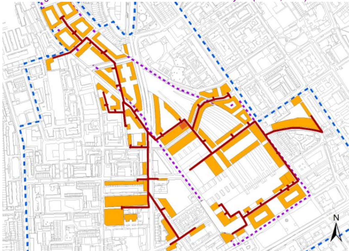
Figure 13.3: Potential Euston area heat network layout (ARUP, 2013)
